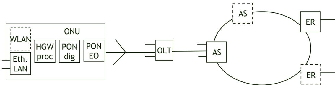
**Figure 6: Wireline access and metro aggregation network with main subsystems considered in the Green Meter. At the optical network unit (ONU): Ethernet local area network (LAN), home gateway processor (HGW proc), passive optical network (PON) digital electronics (digital) and electro-optical transceiver (EO). In the network: optical line termination (OLT), aggregation switch (AS) and edge router (ER).**
