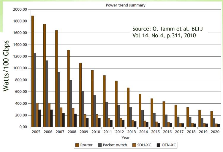
SDH—Synchronous digital hierarchy OTN—Optical transport network XC—Cross-connect
